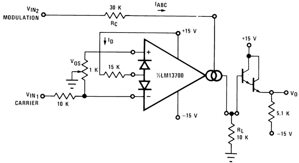
**FIGURE 5. Amplitude Modulator**
